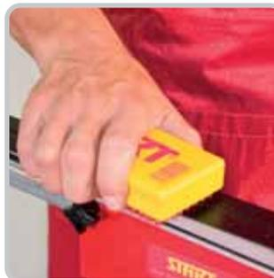
3. Let the base cool down, brush slightly with finishing brush and polish with fibertex.
