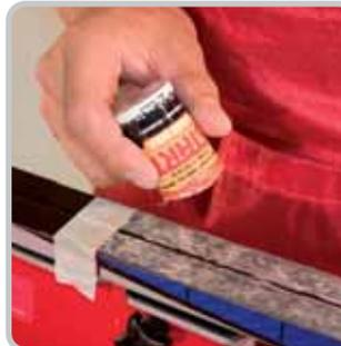
1. Spread layer of base wax on to the base.
