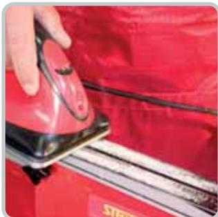
2. Melt the powder with the waxing iron until the wax forms into a smooth layer on the base surface.
