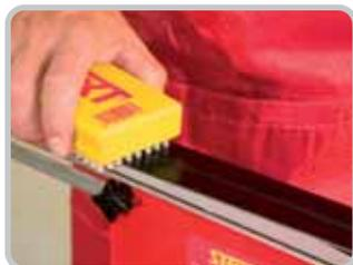
Spread liquid glider on to the pre-prepared gliding base. Let dry well and remove extra wax carefully by brushing.
