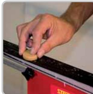
1. Apply thin layer of block glide waxed base
