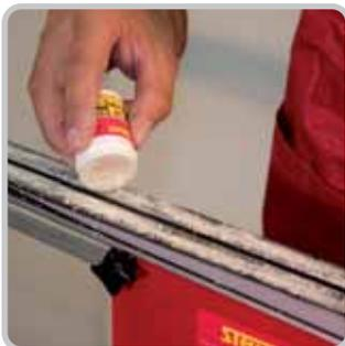
1. Spread even layer of powder on to the pre-prepared base surface.
