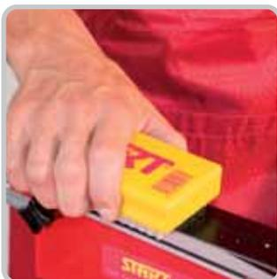
3. Let cool down and remove extra wax by brushing with nylon and finishing brush.
