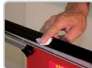
1. Apply the Accelerator liquid on to the gliding base. Note! Only 2-3 drops for entire base both sides of the groove.
