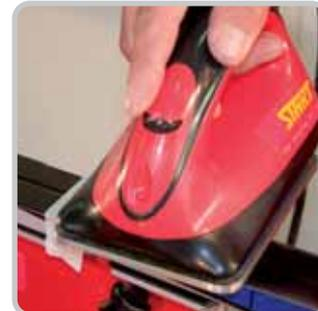
2. Fasten the Base-wax with iron on to the base.
